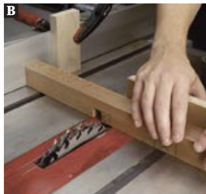
B For the second pass, butt the workpiece against the fence. This doubles the dado width without a setup change.
